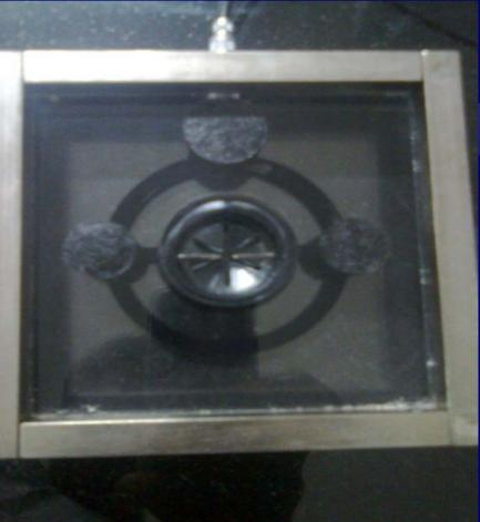
Test piece is placed on filter papers
