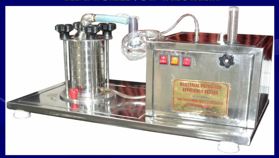
This instrument measures the percent efficiency at which the face mask filters bacteria passing through the mask.
