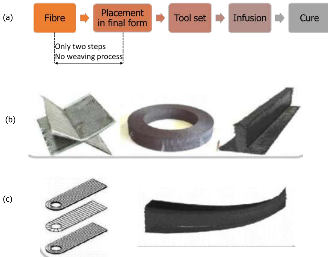
Figure 28.18 (a) Process flow of "D3D" process (b & c) Final products prepared by this method
